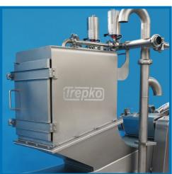
The homogenizer enable a continuous processing of the product and can be offered in a fully automatic version, which ensure that no excess-kneading occur. In addition this version allow the system to communicate with the upstream TREPKO 861 Block Chopper and the downstream filling machine insuring that product is supplied at a continuous and adequate speed safeguarding the entire line from stops due to overflow or missing product.
