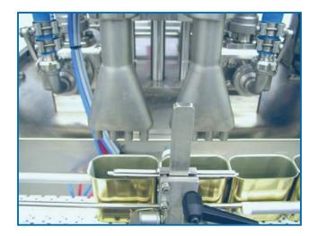
The 620 Series also includes filling machines equipped with slat conveyors for container supply and collection. One example of this setup include units with scrolls for transportation of glass jars. Depending on the production size these filling systems are designed with between one and eight filling heads, while the glass jars are moved in either one or two lane batches.
