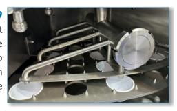
Additionally the machine features a cup leakage test function that detects any leaks from the membrane lid, the seal or the cups. In the event of a defective package, the machines built-in function for disposal removes it, thereby further enhancing the safety and reliability of your production line.
