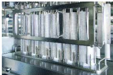
ergonomic cup stack feeding magazine
